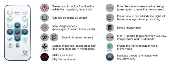
Important: for the remote to function effectively, ensure it is used in close proximity to the lamp's camera. Additionally, point the remote directly towards the camera for better signal reception.
